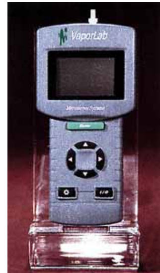
Photo 2. A commercially available handheld SAW chemical vapor analyzer incorporates an array of four SAW sensors, each coated with a different polymer.
