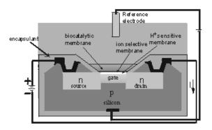
Figure 1A sketch showing the operation of an ENFET where ion sensitive membranes setup a potential difference which controls the gate bias and consequently the channel conductivity between the source and drain.
