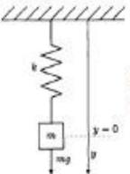
Mass-Spring System with Hardening Spring (simple nonlinear mechanical system)
