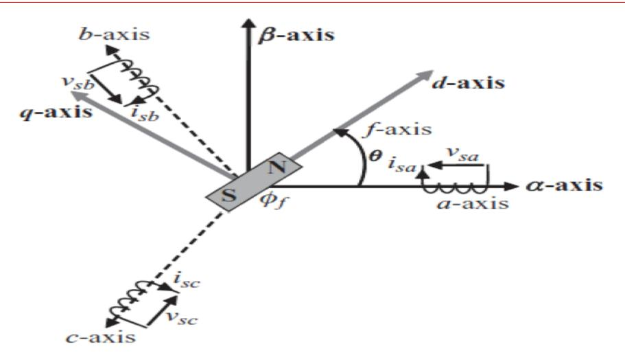
The Three-Phase *abc*-Coordinate Frame, The  $\alpha\beta$  Stationary Two-Phase Coordinate Frame, and the *dq* Rotating Two-Phase Coordinate Frame for the PMSM
