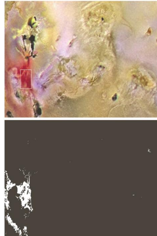
FIGURE 6.44 Segmentation in RGB space. (a) Original image with colors of interest shown enclosed by a rectangle. (b) Result of segmentation in RGB vector space. Compare with Fig. 6.42(h).
