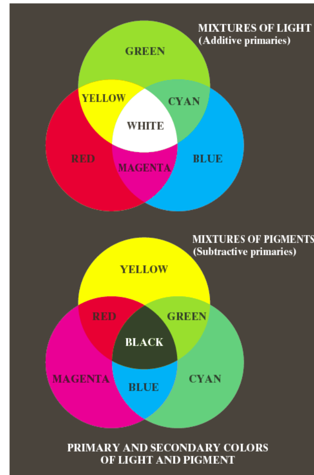
FIGURE 6.4 Primary and secondary colors of light and pigments. (Courtesy of the General Electric Co., Lamp Business Division.)
