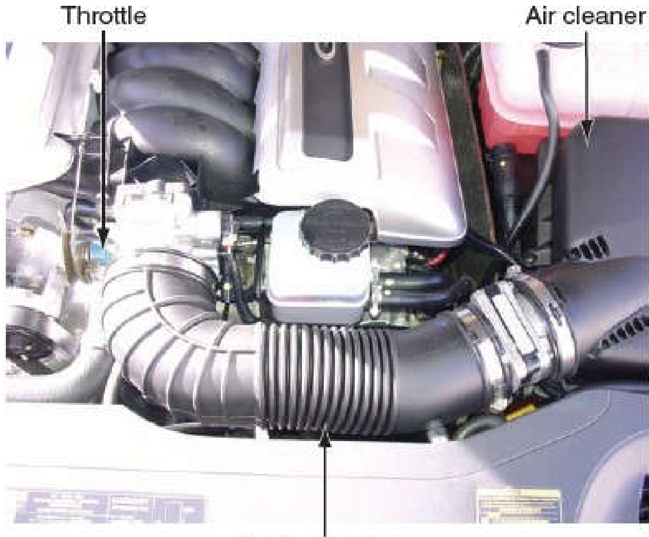
Figure 50.1 Remove the air cleaner and hose. Be careful not to crack the hose.
